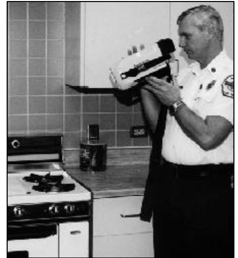
Lt. Richard Wydra aims one of the Village's two thermal-imaging cameras at a gas-stove burner. What he sees in the viewfinder reveals any heat source and even provides a readout of the source's temperature.
